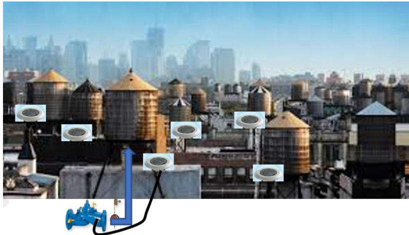
Cellular pressure transmitter installed on a fire reserve tank fill control valve to monitor fire reserve tank level
